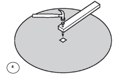
c. Put a carpenter's level on the wood plank and swing the board in a circle to find the high and low spots. (Image 5)
