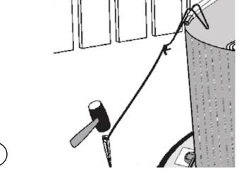
d. When uncoiling the wall, the skimmer and return holes are positioned toward the end of the wall. (Image 4)
