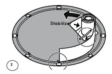
c. Set lengths of stabilizer onto the top edge of the wall as you uncoil it. (Image 2)
